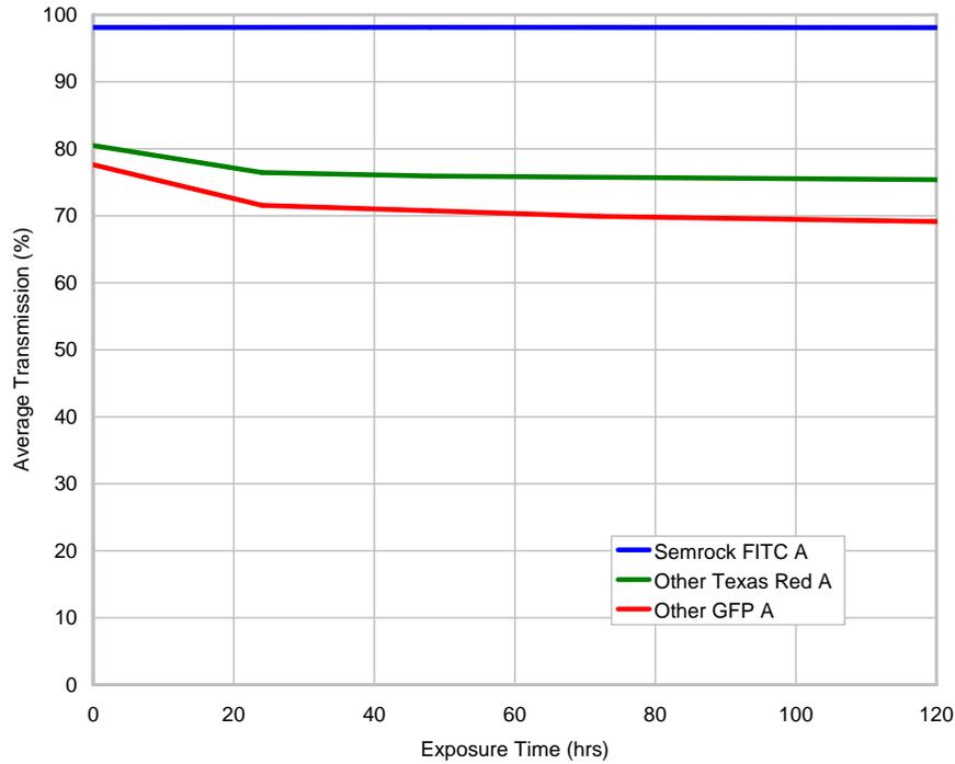
**Figure 14:** Measured average transmission over the passband of the “Other GFP A,” “Other Texas Red A,” and “Semrock FITC A” filters. The Semrock filter shows no change.
