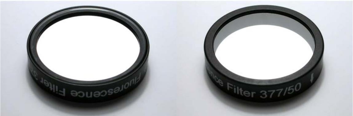
**Figure 10:** Photographs of both sides of the “Semrock DAPI B” filter after about 500 hours of exposure to 6W of total power over a 25 mm diameter. The filter showed no signs of degradation.
