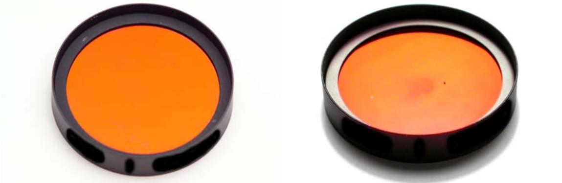
**Figure 8:** Photographs of the “Other DAPI B” filter before and after about 500 hours of exposure to 6 W of total power over a 25 mm diameter. The dig defects and apparent “burning” are real.
