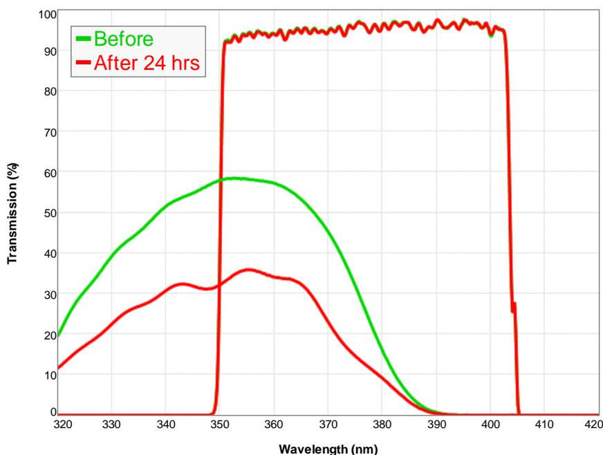
**Figure 1:** Transmission spectra of “Other DAPI A” (lower left spectra) and “Semrock DAPI A” (upper right spectra) filters before (green) and after (red) exposure to 15 W of total power for 1 day.
