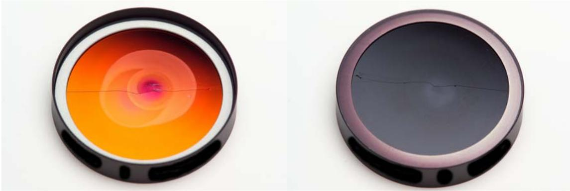
**Figure 2:** Photographs of both sides of the “Other DAPI A” filter after about 300 hours (just over 12 days) of exposure to first 15 W (1 day) and then 2.5 W of total power. Note severe discoloration in the most intense region of exposure as well as a severe crack that extends across the entire filter through both sides.
