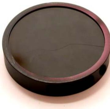
**Figure 9:** Photograph of the “Other DAPI C” filter after about 300 hours of exposure to 6 W of total power over a 25 mm diameter. At this point it developed a severe crack which allows light to leak through the filter.
