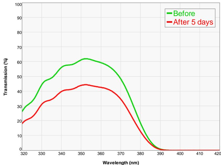
**Figure 4:** Measured transmission spectra of the “Other DAPI B” filter before exposure and after 5 days.
