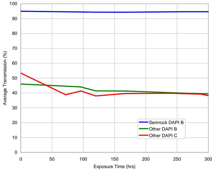
**Figure 7:** Measured average transmission over the passband of the “Other DAPI B,” “Other DAPI C,” and “Semrock DAPI B” filters. The fluctuations in transmission of the “Other” filters are believed to be real, and do not result merely from measurement error.
