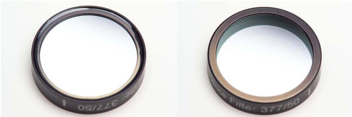
**Figure 3:** Photographs of both sides of the “Semrock DAPI A” filter after over 1000 hours of exposure to first 15 W (1 day) and then 2.5 W of total power. The filter looks identical to its appearance before exposure.
