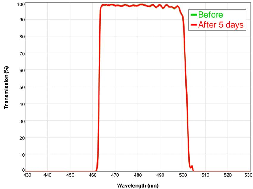
**Figure 13:** Measured transmission spectra of the “Semrock FITC A” filter before exposure and after 5 days. The filter exhibited no measurable change.
