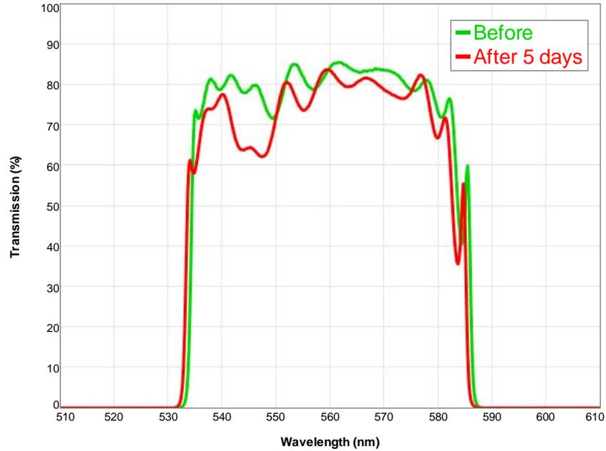
**Figure 12:** Measured transmission spectra of the “Other Texas Red A” filter before exposure and after 5 days. This filter exhibited a blue shift and a significant change in the passband ripple, resulting in a loss of average transmission.
