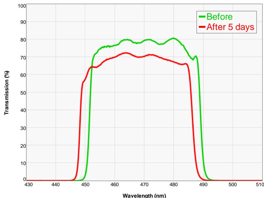
**Figure 11:** Measured transmission spectra of the “Other GFP A” filter before exposure and after 5 days. Note the significant loss of transmission and blue shift of the spectrum.
