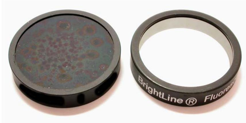
**Figure 16:** Photographs of the filters “Other DAPI D” (left) and “Semrock DAPI C” (right) after 10 x 24 hour cycles of aggravated humidity testing according to the MIL-STD-810F. Note the significant degradation of the “Other” filter. The Semrock filter showed no apparent change in appearance.
