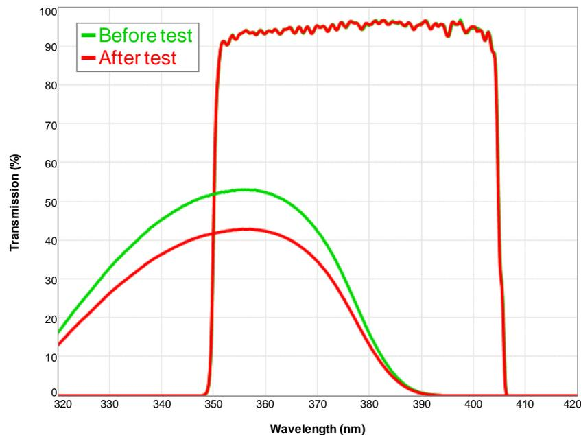
**Figure 17:** Transmission spectra of “Other DAPI D” (lower left spectra) and “Semrock DAPI C” (upper right spectra) filters before (green) and after (red) 10 x 24 hour cycles of aggravated humidity testing according to the MIL-STD-810F. Note the significant decrease in transmission of the “Other” filter. The Semrock filter did not exhibit any measurable spectral change.
