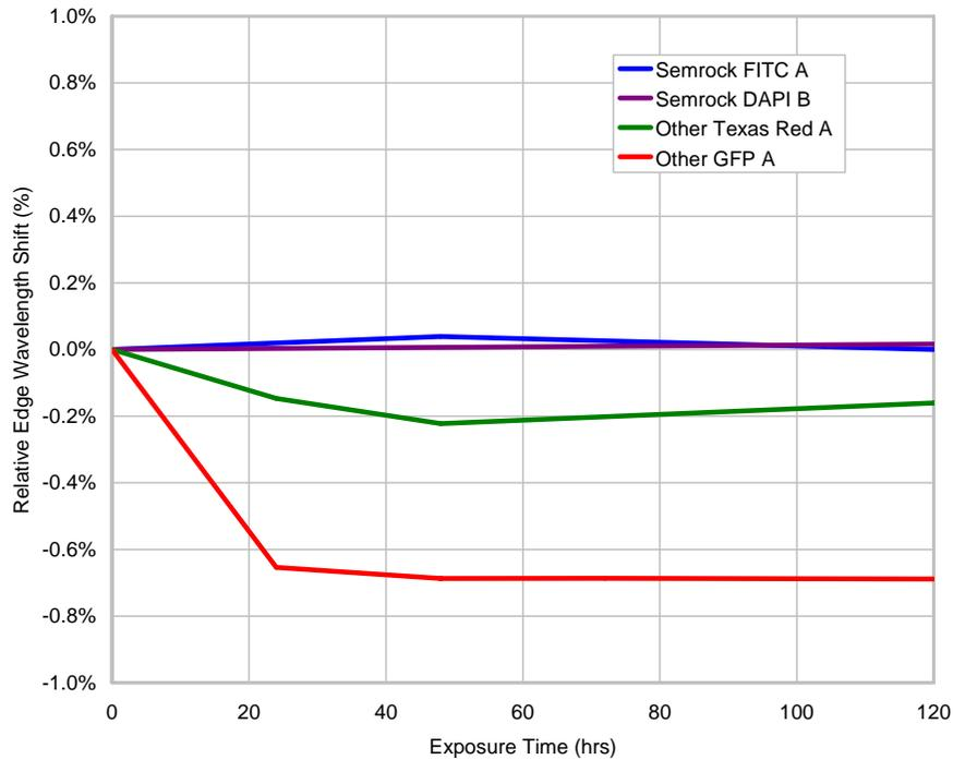
**Figure 15:** Measured wavelength shift of the short-wavelength edge on the “Other GFP A,” “Other Texas Red A,” “Semrock FITC A,” and “Semrock DAPI B” filters.
