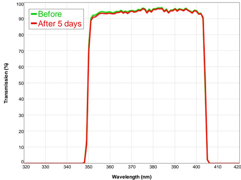
**Figure 6:** Measured transmission spectra of the “Semrock DAPI B” filter before exposure and after 5 days. The slight decrease in transmission is believed to be a measurement artifact, as it later increased again.
