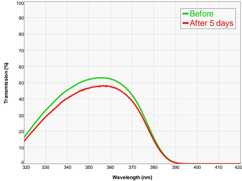
**Figure 5:** Measured transmission spectra of the “Other DAPI C” filter before exposure and after 5 days.
